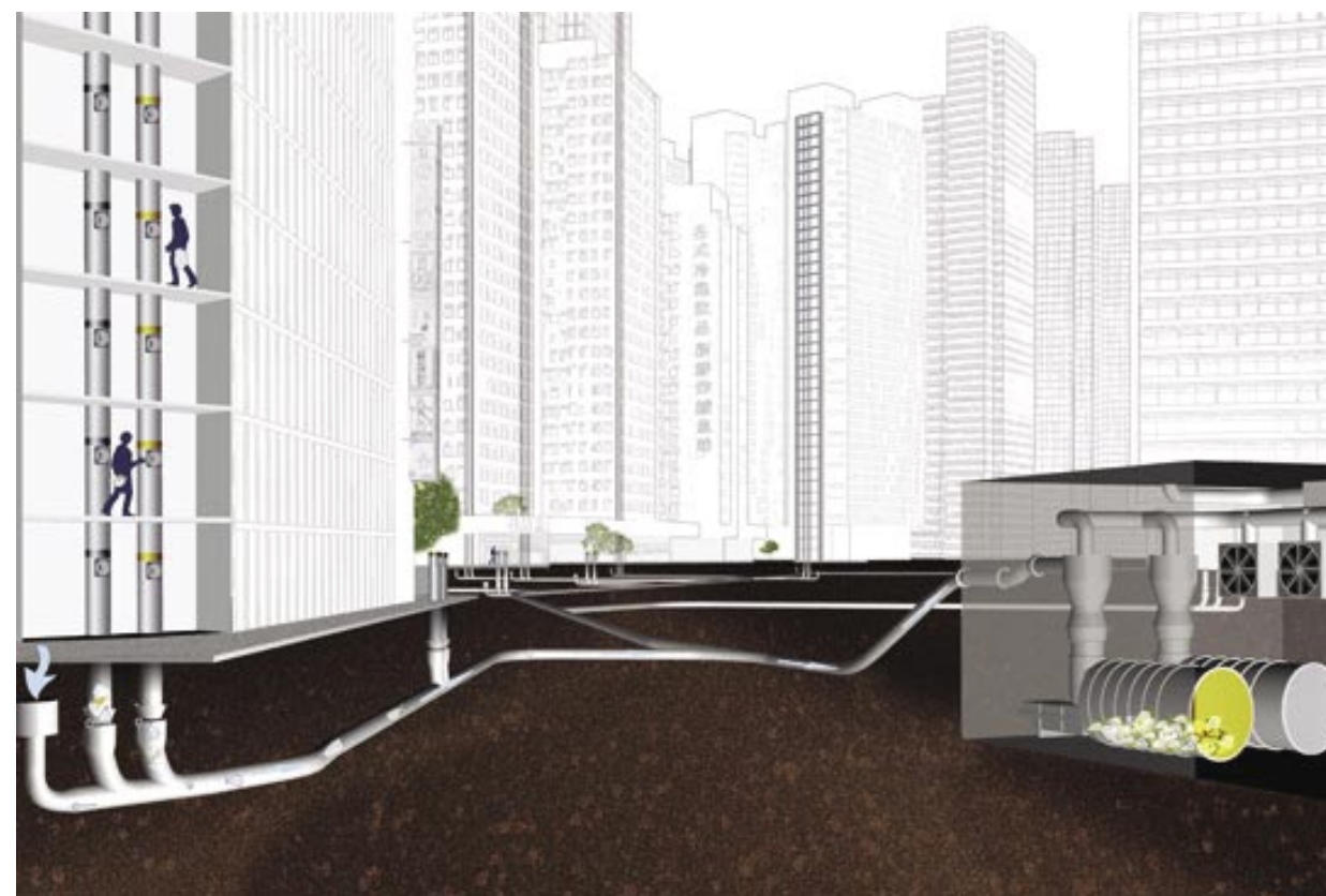
ENVAC Waste Disposal System
