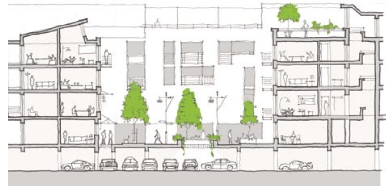
Typical section through courtyard
